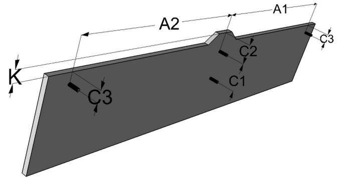
**A1, A2:** Measure the distance along the outside of the saxboard from center of bolt to center of bolt
